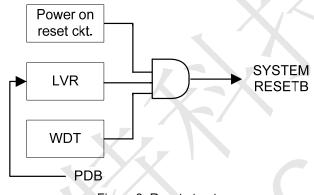
Figure 3: Reset structure
